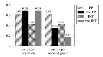
Fig. 1. Energy consumption in nanojoules (nJ) per FMA (including necessary L1 loads and stores) and per group of operands for vectorized and non-vectorized double-precision floating point and integer loads.
