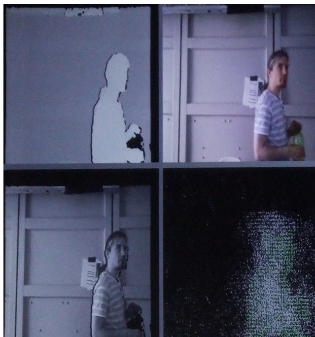
Figure 12: Visualization of the images captured by the Kinect camera with a person passing by. The top left shows the image captured by the depth sensor, the top right the image captured by the normal sensor. The bottom left is a masked version of this image (in this case the entire scene is in range and hence visible) and the bottom right shows the captured motion information.
